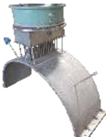
20 KW Indirect Chemical reactor with Flame Proof Enclosure
